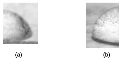
Figure 4. (a) Water droplet on untreated Teflon film. (b) Water droplet on Teflon film, treated with compound 6 (Note changes in contact angle of droplet between a and b).
